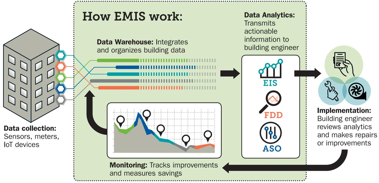
**EMIS TOOLS:** Energy information systems (**EIS**) help find energy waste using smart meter data. Fault detection and diagnostic tools (**FDD**) detect and prioritize HVAC system faults. Automated system optimization (**ASO**) includes control algorithms to minimize energy use across systems.
